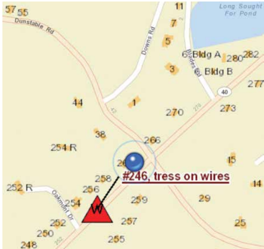
The town of Westford uses its GIS system as a backbone for its real-time damage assessment data. Town employees can view problems on their smartphones.
