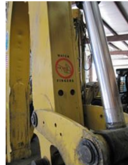
Worker's finger entered an observation hole on the boom and was sliced by the piston.
