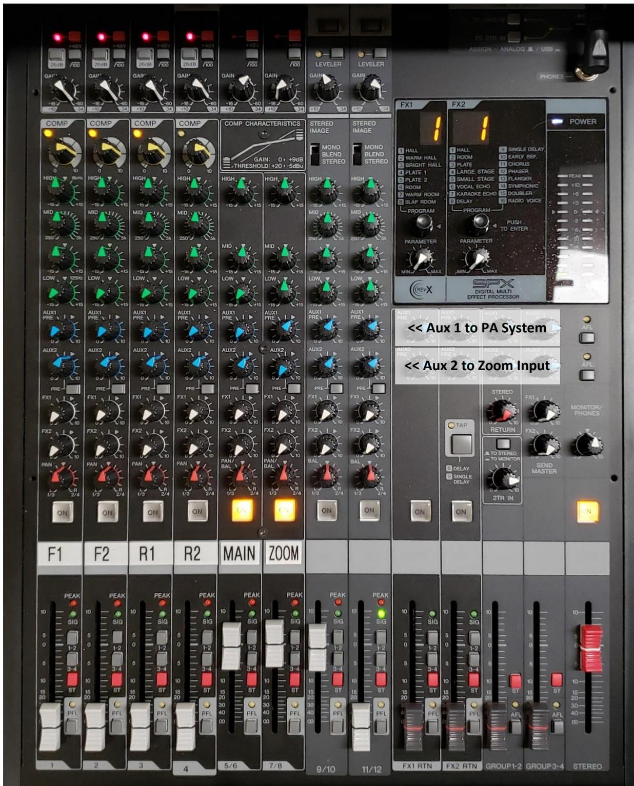
The Yamaha mixer for program feeds to the recorders and cable channel/stream. The blue dials indicate the settings for the Aux 1 and Aux 2 sub-mix audio feeds.
