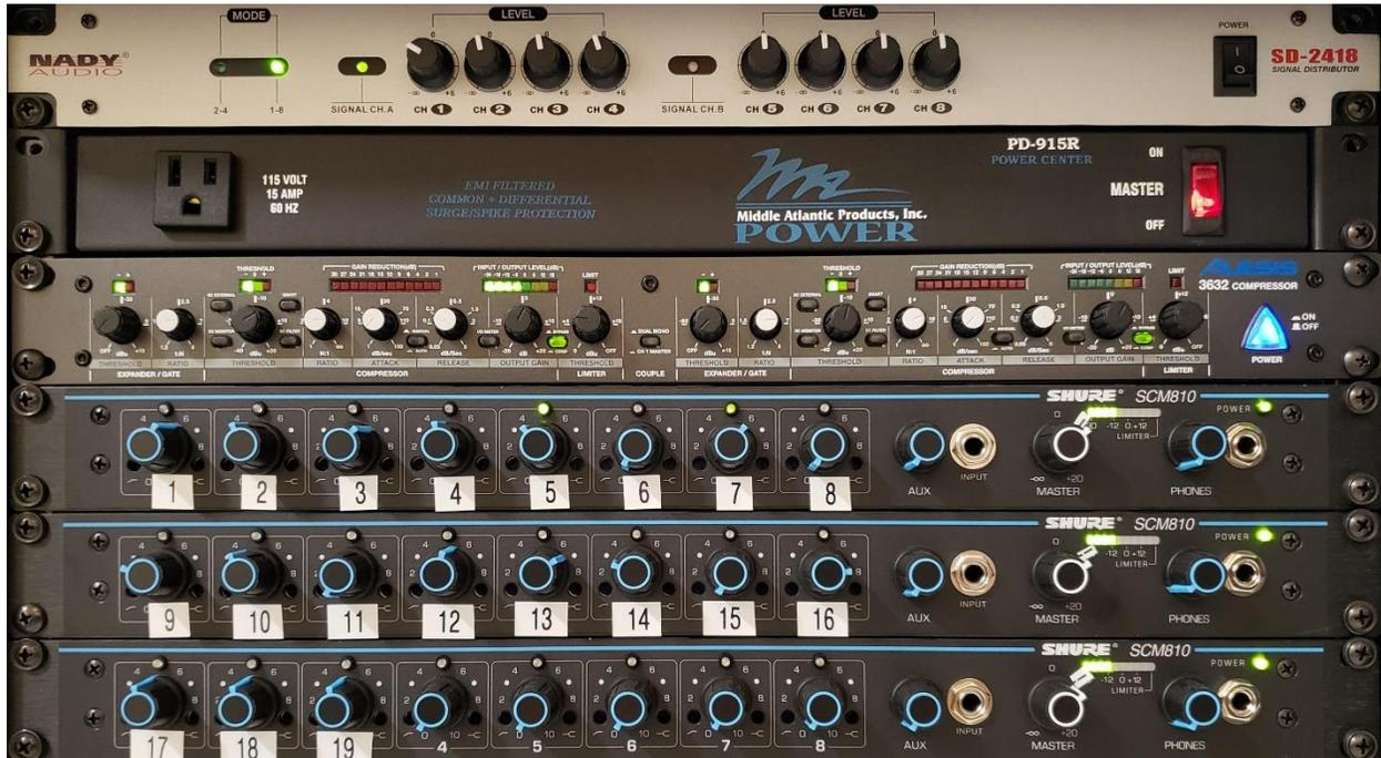
The Nady distribution amplifier sends the mixed microphones to the Chambers P.A. system, the Yamaha Program mixer (via the compressor) and to a dedicated microphones level meter.
