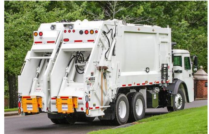
Depiction of Split trucks that are used to allow pick-up of trash and recycling in one vehicle
