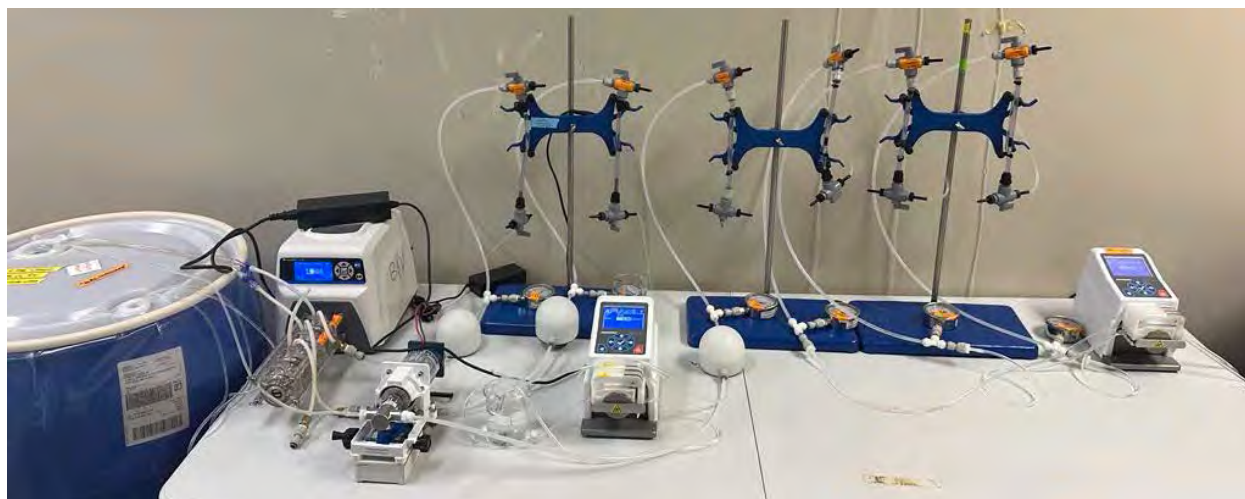
Figure 3-2 RSSCT Bench-Scale Testing Experimental Setup (55-gallon drum of feed water on left, pumps, and RSSCT columns mounted on stands with valves and flow measurement)
